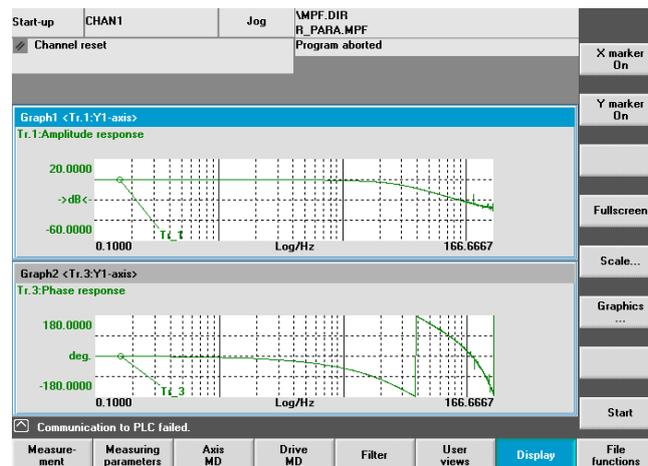
Figure 11-6 Optimized position control loop
