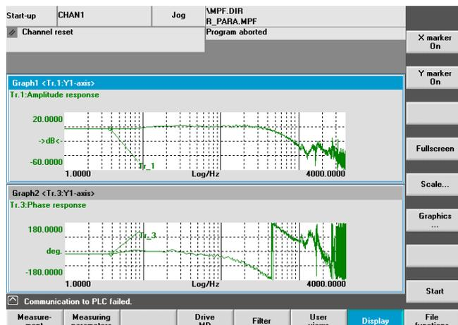
Figure 11-5 Optimized speed control loop
