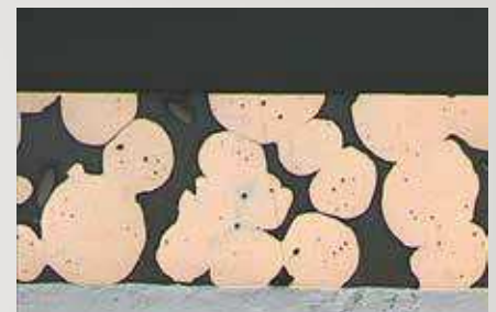
Fig. 8: Condition of sliding surface during service life
