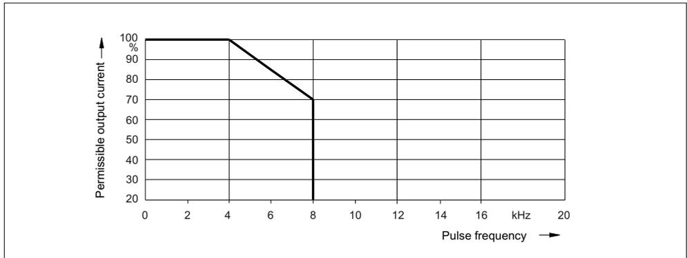
Figure 3-27 Frame size FSF: Output current as a function of the pulse frequency
