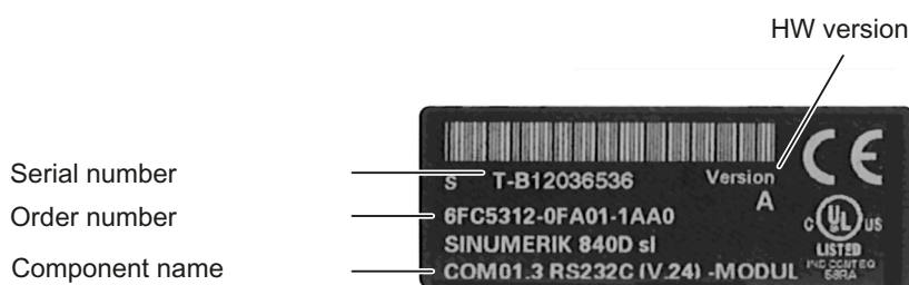
Figure 9-21 COM01.3 RS 232C (V.24) module type plate
