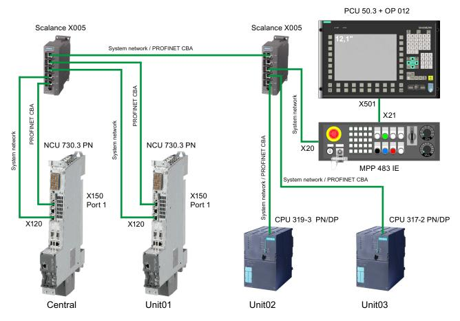
Figure 7-8 Example PROFINET CBA configuration
