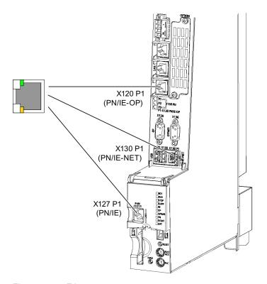
Figure 7-5 Ethernet ports
