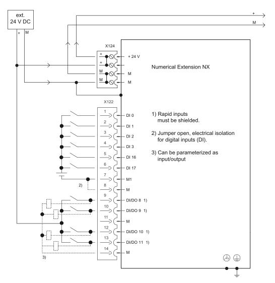
Figure 9-6 Block diagram for digital inputs/outputs
