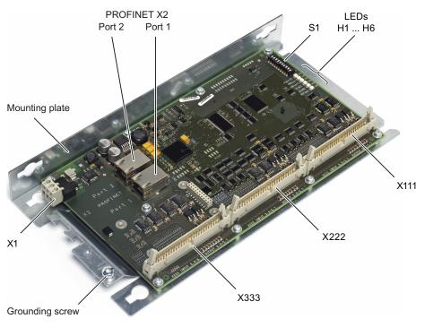
Figure 9-7 PP 72/48D PN I/O module
