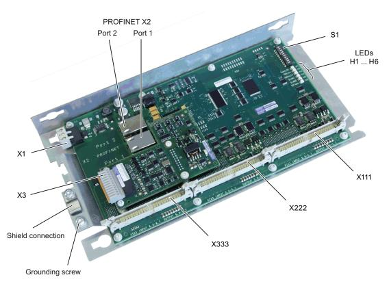
Figure 9-13 PP 72/48D 2/2A PN I/O module
