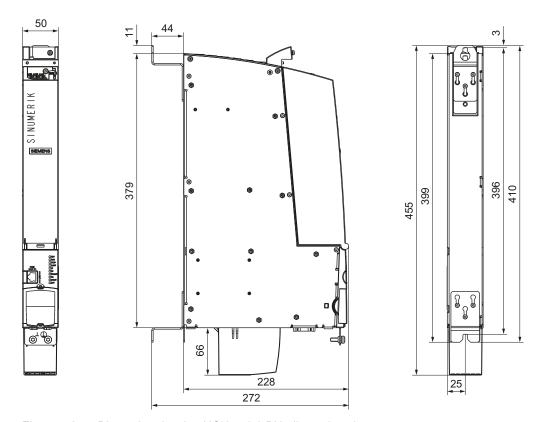
Figure 5-2 Dimension drawing NCU 710.3 PN; dimensions in mm
