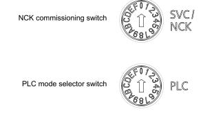
Figure 3-5 Startup and mode selector switch
