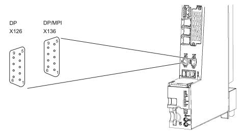
Figure 7-9 PROFIBUS DP/MPI interfaces
