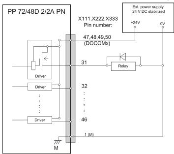
Figure 9-18 Terminal assignment for the digital outputs
