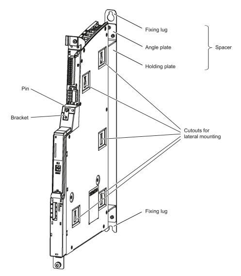
Figure 9-4 Mounting aids for the NX module
