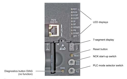
Figure 3-4 Position of operator control and display elements
