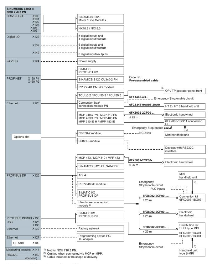
Figure 7-1 Options of connecting an NCU
