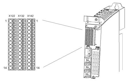
Figure 7-11 Digital inputs/outputs (interfaces X122, X132 and X142)
