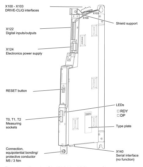
Figure 9-1 Illustration of the NX10.3 / 15.3 (without cover)
