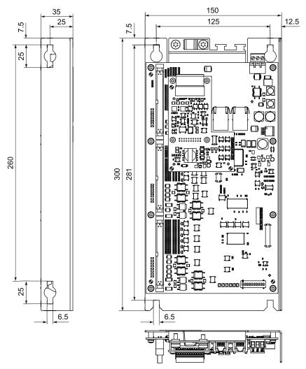
Figure 9-15 PP 72/48D 2/2A PN dimension drawing
