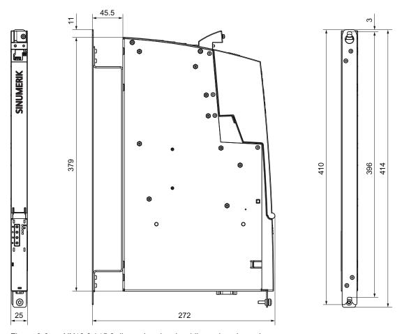
Figure 9-3 NX10.3 / 15.3 dimension drawing (dimensions in mm)
