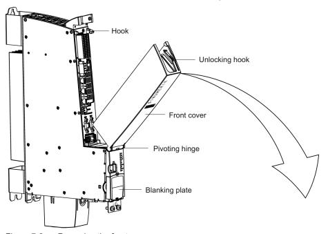
Figure 7-2 Removing the front cover
