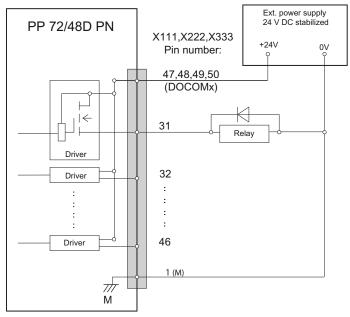
Figure 9-12 Terminal assignment for the digital outputs
