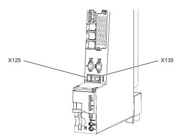
Figure 7-14 Position of USB interfaces
