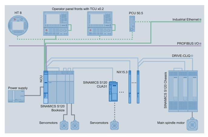
Figure 2-1 Typical topology of the SINUMERIK 840D sl complete system
