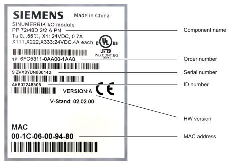
Figure 9-14 PP 72/48D 2/2A PN type plate
