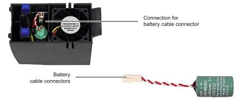
Figure 10-1 Battery replacement in the dual fan/battery module
