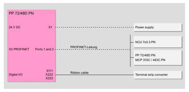
Figure 9-10 I/O module connection options
