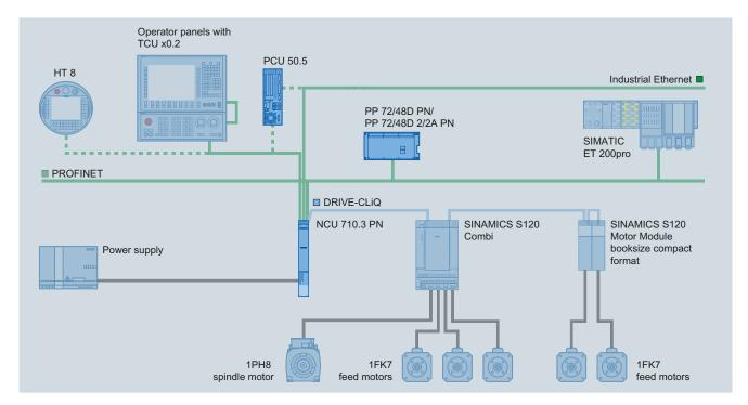
Figure 2-2 Sample topology which is only possible with an NCU 710.3 PN
