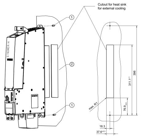
Figure 6-1 Panel cutout (dimensions in mm)
