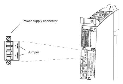
Figure 7-3 Power supply interface
