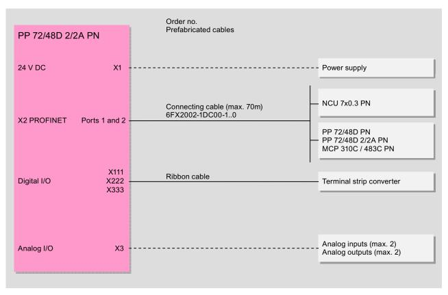
Figure 9-16 Connection options of the PP 72/48D 2/2A PN I/O module
