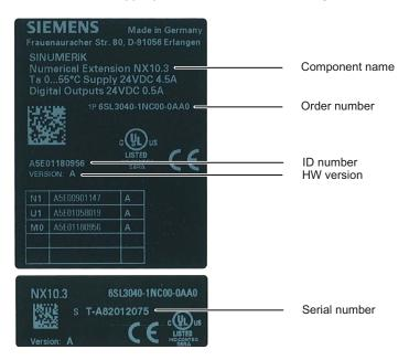
Figure 9-2 Type plate using the NX10.3 as example
