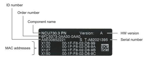
Figure 3-3 MAC addresses of the PROFINET/Ethernet interfaces
