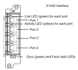
Figure 9-23 CBE30-2 Ethernet communication board
