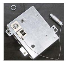
2. Attach the bracket for the terminating connector.
