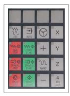
Figure 17-23 HT2 slide-in labels
