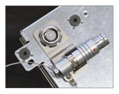
**3.** Tighten the retaining nut and insert the terminating connector into the bracket.
