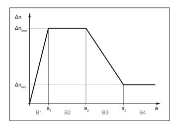
$\begin{array}{ll} \Delta n_{\text{max}} & \text{Maximum compensation value} \\ \Delta n_{\text{min}} & \text{Minimum compensation value} \end{array}$
