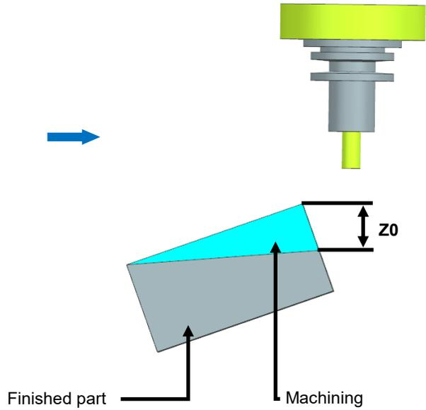
The values for the traversal paths are calculated with the angle functions.
