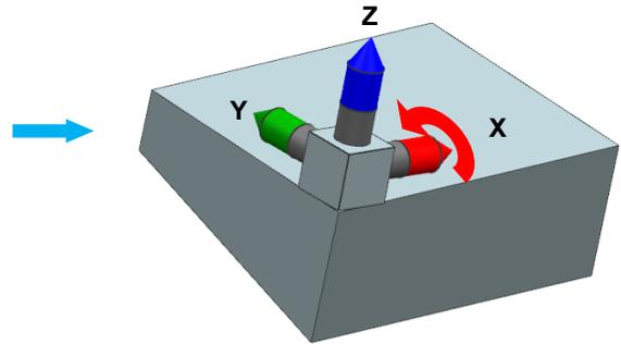
The face cutting in the swivel plane follows. A protrusion  $>100$  mm is programmed in "X1" and "Y1" so that no edge remains.
