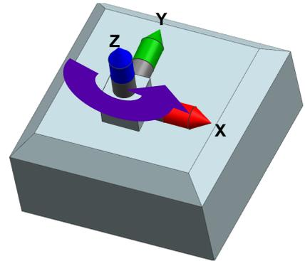
Beta specifies the rotation angle in space (rotation at the new Y axis).
