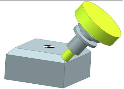
In the "END" block, "CYCLE800" travels to the initial setting and the Tool Carrier is deselected.
