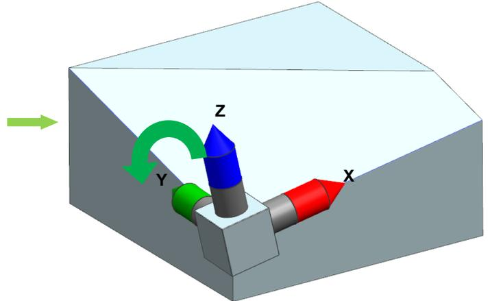
The surface can be programmed only via projection angles, but not via axis angles.
