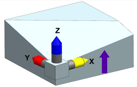
the second projection angle "Yα" is programmed. This is the angle by which the Y axis must be rotated so that the shown component edge results.
