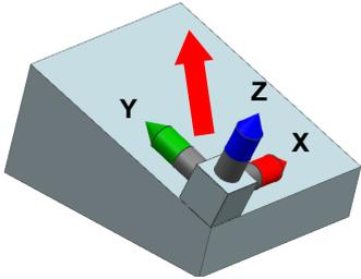
If swiveling requires that the position of the coordinate system is moved, this is performed for each axis via the **X0**, **Y0** and **Z0** parameters.
