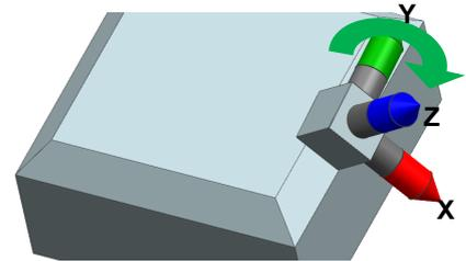
In the **first** step, the coordinate cross is moved to the swivel point (chamfer start).
