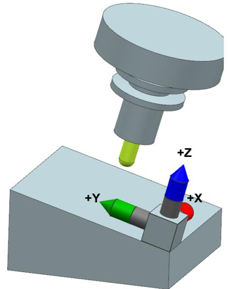
The input screen of "CYCLE800" represents the machine kinematics.
