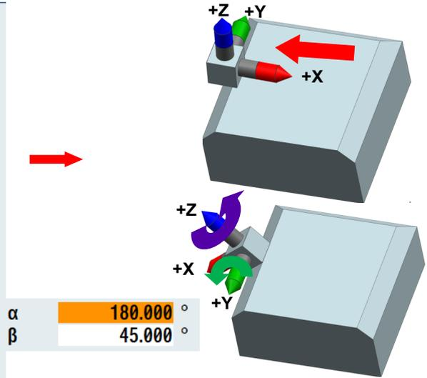
The third chamfer is programmed in the "3\_CHAMFER" block.
