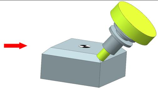
In the "END" block, "CYCLE800" travels to the initial setting and the Tool Carrier deselected.
