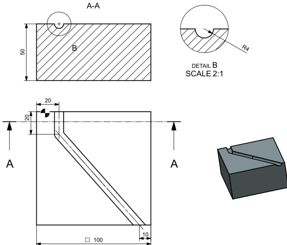
The tool orientation is always perpendicular to the machining plane after swiveling with "CYCLE800".
