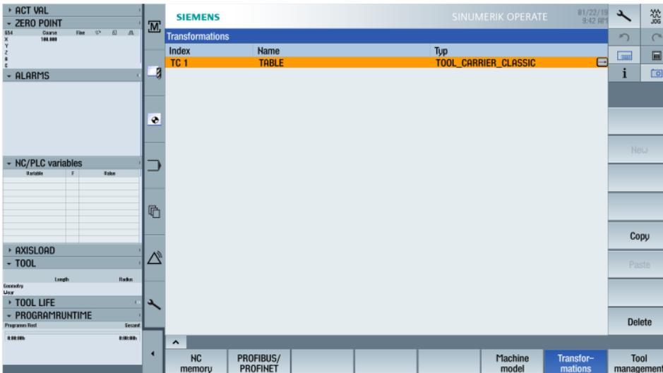
opens the Tool Carrier. The name of the TC ("TABLE") is arbitrary. If necessary, several Tool Carriers can also be created, for example, when a replaceable head is used for machining.
