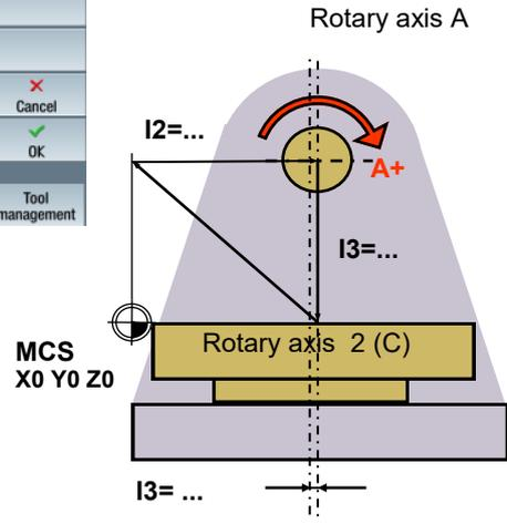
In addition to the values for the axis measurement, machine-related strategies are also specified in the Tool Carrier. Such strategies are normally made by the machine manufacturer / distributor.
