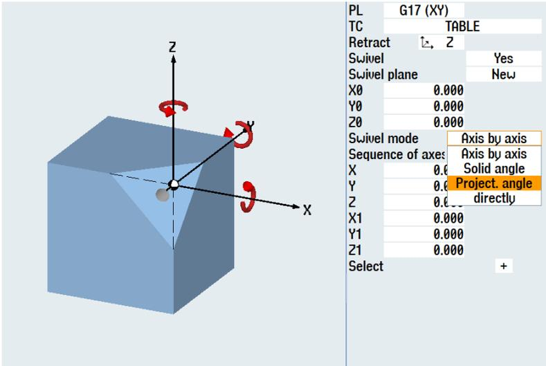
In the first step, move the coordinate cross to the swivel point (chamfer start).
