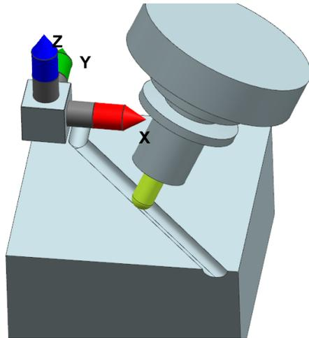
the tool can be set at the "X" and "Y" axes.
