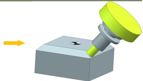
In the "END" block, "CYCLE800" travels to the initial setting and the Tool Carrier is deselected.
