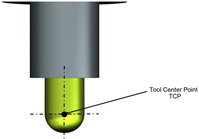
Once the ball mill has been measured in this way, it can be swiveled arbitrary at the point or "set". In the simulation, only the external diameter of the tool is represented as cutter.
