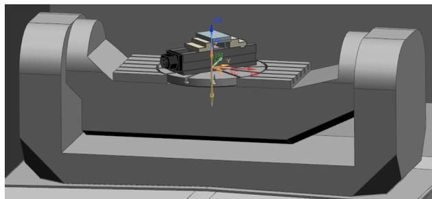
With the "additive" swivel plane, the following swiveling adds to the previous one.
