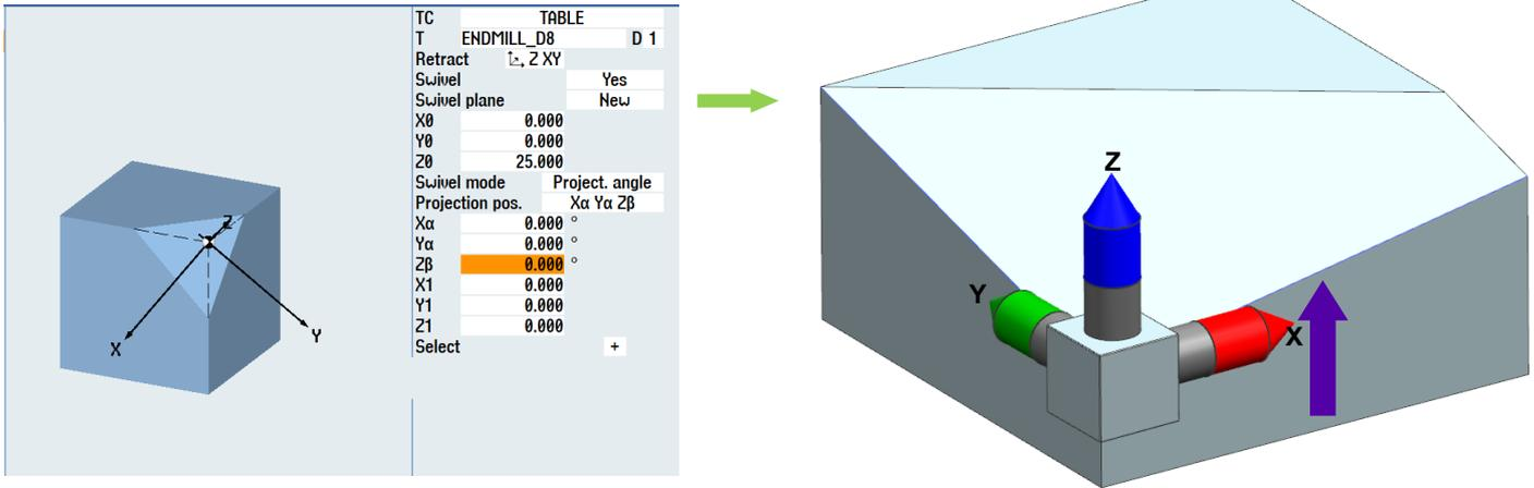
"Xα" is the angle by which the X axis must be rotated so that the component edge results in the Y/Z plane.
