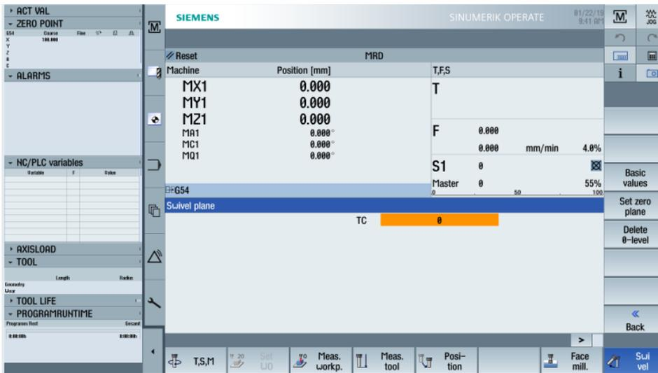
If no TC (Tool Carrier) that contains the machine kinematics for swiveling is selected, this field remains empty.
