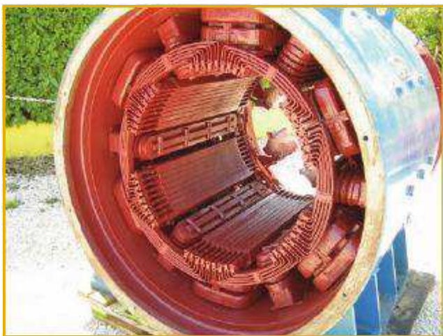
Motor C.C. 1500 Kw. 600 Volts after dryer to the oven
