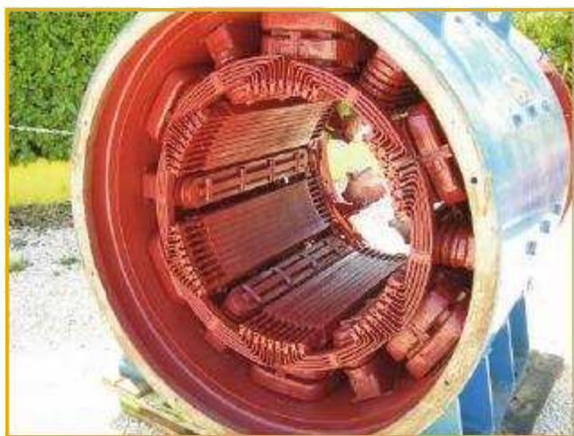
Motor C.C. 1500 Kw. 600 Volts after dryer to the oven
