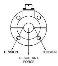
NOTE: If the orientation of the sensor requires the force direction arrow to be pointed opposite the resultant tension force direction, then the black (-S) and the white (+S) sensor leads to the MAGPOWR readout or control terminal block must be reversed.
