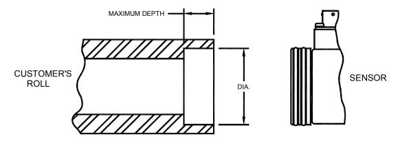
$52.0_{-.00}^{+.05}$  mm diameter; 0.53 in. (13.5 mm) maximum depth for 5 lb, 50 lb, 2 kg, & 25 kg sensors  $62.0_{-.00}^{+.05}$  mm diameter; 0.76 in. (13.9 mm) maximum depth for 150 lb, 500 lb, 75 kg, & 250 kg sensors
