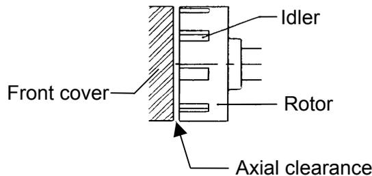
Figure 31: The axial clearance between the rotor/idler and the front cover.
