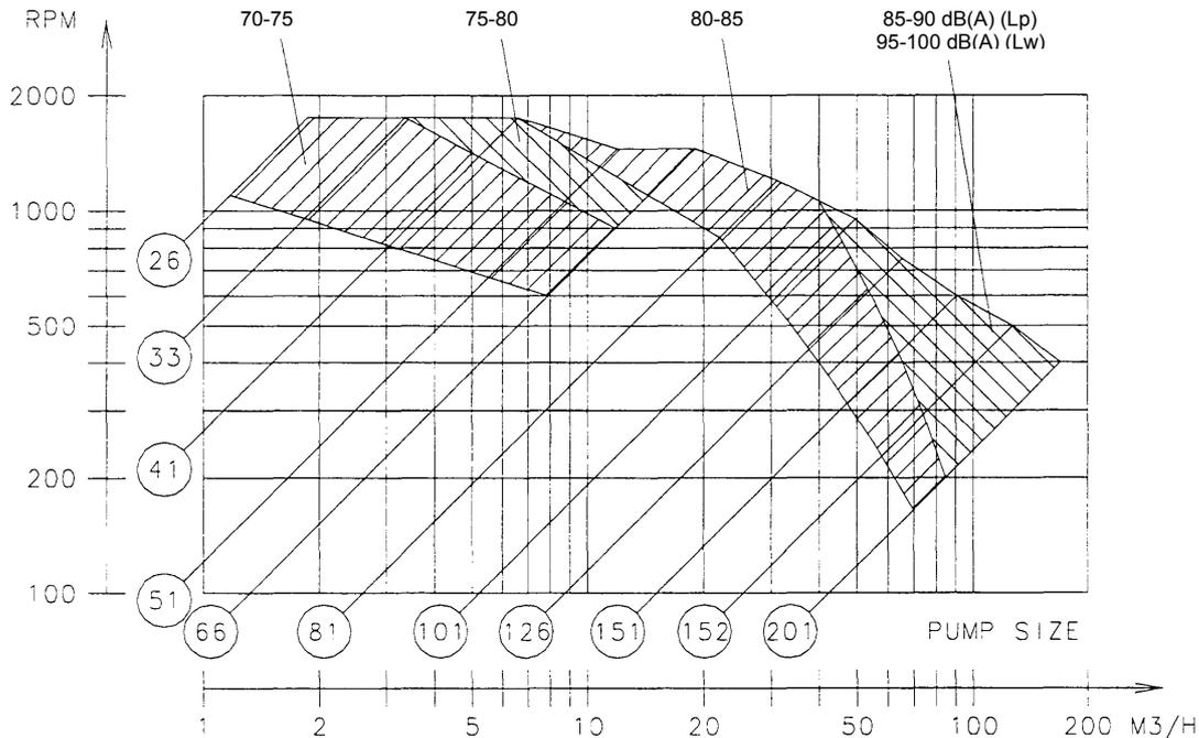
Figure 22: The maximum A-weighted sound pressure level in dB(A)(Lp) for the various pump sizes in relation to the pumps' flow. The range above 85 dB(A) is also expressed as sound power level (Lw).
