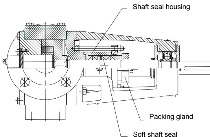
Figure 24: The location of the soft shaft seal, the shaft seal housing and the packing gland on the pump. The design of the shaft seal housing, does, however, depend on the individual pump application.
