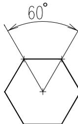
Figure 35: The size of the angle for a single surface on the hexagonal bolt head on the adjusting screws.
