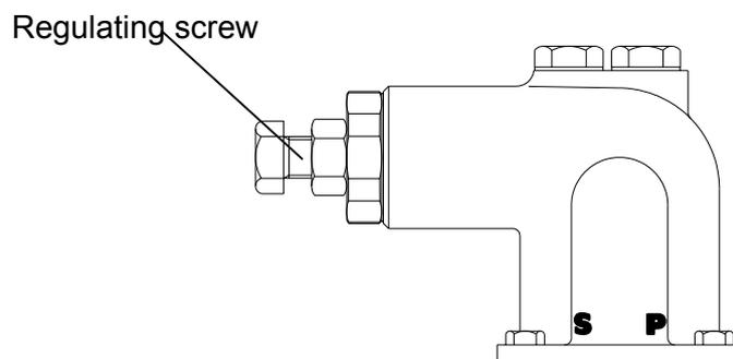
Figure 17: The location of the regulating screw on the ROTAN safety valve.
