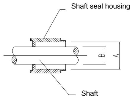
Figure 25: The A and B dimensions on the shaft and the shaft seal housing
