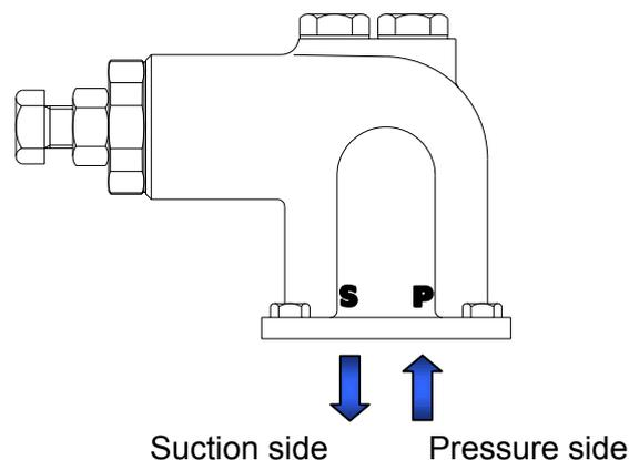
Figure 16: Shows how **S** for suction side and **P** for pressure side are indicated on the valve.
