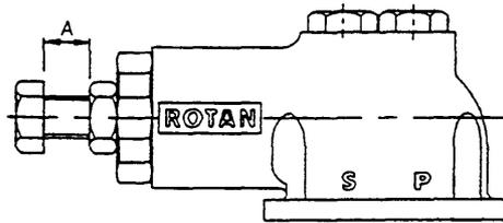
Figure 18: The setting value "A" for ROTAN valves.
