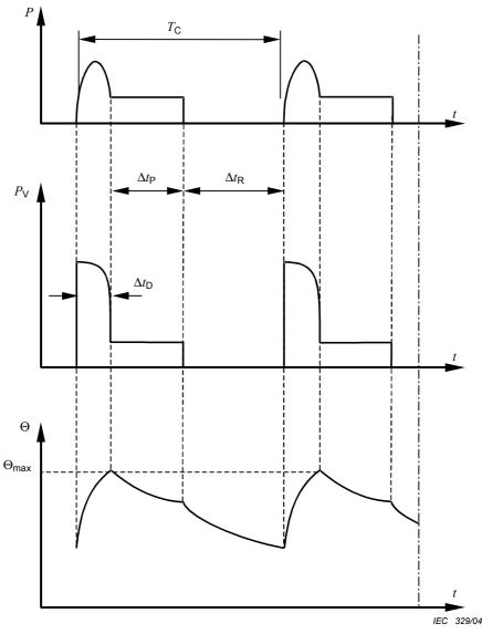
Key P load t time electrical losses  $T_{\mathsf{C}}$ time of one load cycle  $P_{V}$ starting/accelerating time Θ temperature  $\Delta t_{D}$ maximum temperature attained operation time at constant load  $\Theta_{\text{max}}$  $\Delta t_{\mathsf{P}}$ time de-energized and at rest  $\Delta t_{\mathsf{R}}$ Cyclic duration factor =  $(\Delta t_D + \Delta t_P)/T_C$
