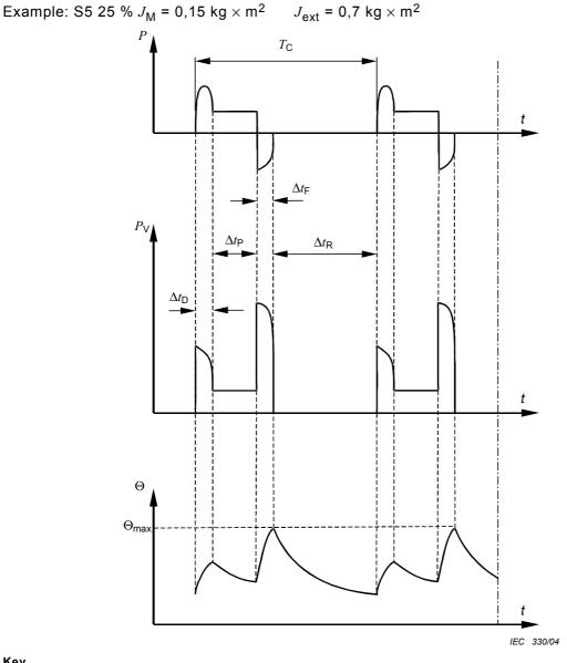
Key load time of one load cycle  $T_{\mathsf{C}}$  $P_{V}$ electrical losses starting/accelerating time  $\Delta t_{\mathsf{D}}$ temperature  $\Delta t_{\mathsf{P}}$ operation time at constant load maximum temperature attained time of electric braking  $\Theta_{\text{max}}$  $\Delta t_{\mathsf{F}}$ time time de-energized and at rest Cyclic duration factor =  $(\Delta t_D + \Delta t_P + \Delta t_F)/T_C$
