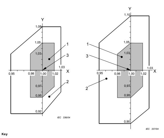
Figure 11 – Voltage and frequency limits for generators
